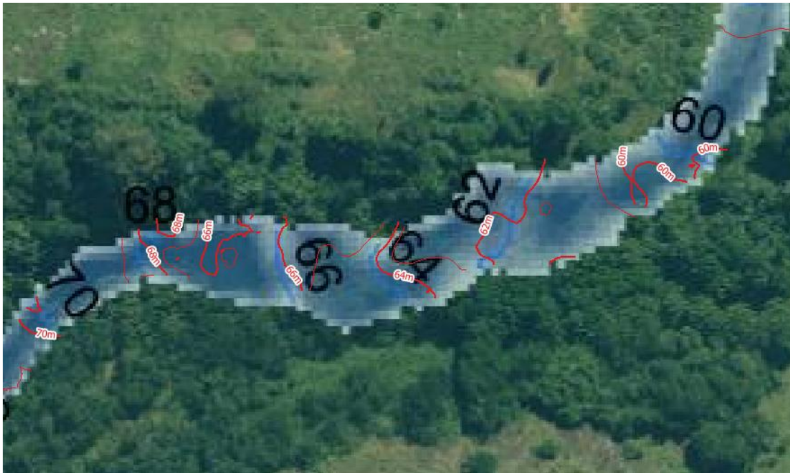
Figure 4-4 Upstream 100 year ARI Flood Level Comparison
